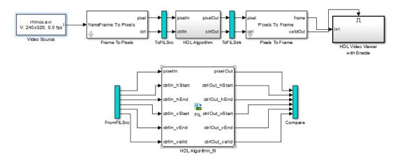
The blue ToFILSrc subsystem branches the pixel-stream input of the HDL Algorithm block to the FromFILSrc subsystem. The blue ToFILSink subsystem branches the pixel-stream output of the HDL Algorithm block into the Compare subsystem, where it is compared with the output of the HDL Algorithm\_fil block. For image and video processing, this setup is slow because the model sends only a single pixel, and its associated control signals, in each packet to and from the FPGA board.
